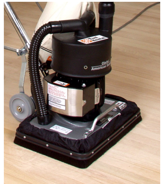
The dust skirt assembly for the OBS 18DC model helps prevent airborne dust.
